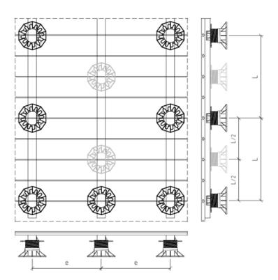
**Step 6:** Using the rooftop flat-top track (for flush against perimeter) begin installing first track against perimeter structure of surface. The patented Mbrico rooftop 4-meter extrusion can be "clicked" into the click top pedestal feet. No additional fastener is required between the extrusion and pedestal. Place pedestals as close to parapet wall as possible on level surface. No greater than 1/3 width of perimeter tile dimension.
