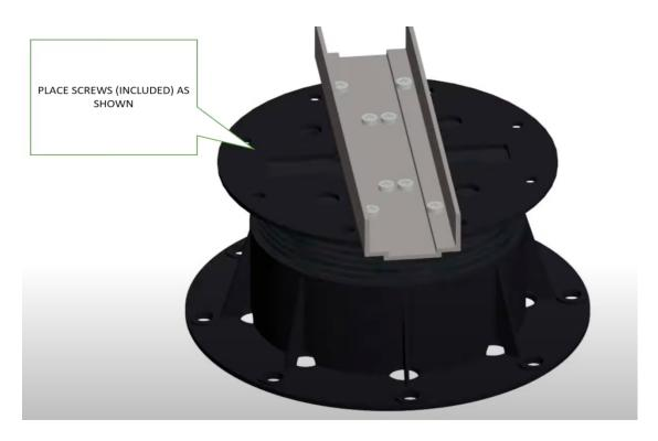
2. Each pedestal with sleeve connector attached will slide into the specific track. Each Pedestal will sleeve connector should be slid into the track prior to tile install. You will slide several pedestals onto each track which can be slide side to side to 24" OC later.
