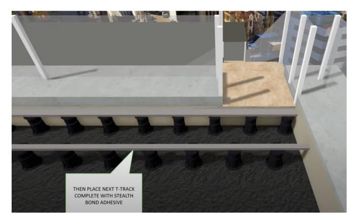
7. Install cross braces to your first track using the supplied cross brace connectors and screws. These are aluminum U-channels that are provided cut to length with all necessary cross brace connectors and screws for attachment.
