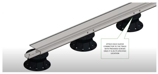
4. To connect two tracks together, slide each track over the sleeve connector & attach with two provided screws per side. There will be 4 total screws on each side of the track end to end connection.
