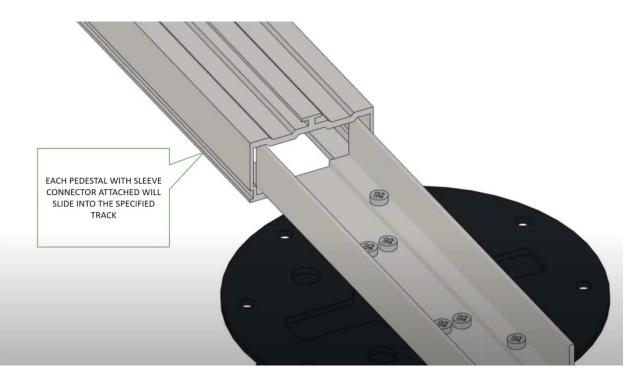
3. Once pedestals are spaced 24" OC according to your Mbrico shop drawing, use provide screws to attach sleeve to track.
