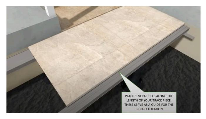
10. Continue adding tile and attaching one end of your cross brace channels until the tile row is complete. Then use a rubber mallet to lock both grooved edges of the tile tightly into the track splines to ensure proper spacing and square.
