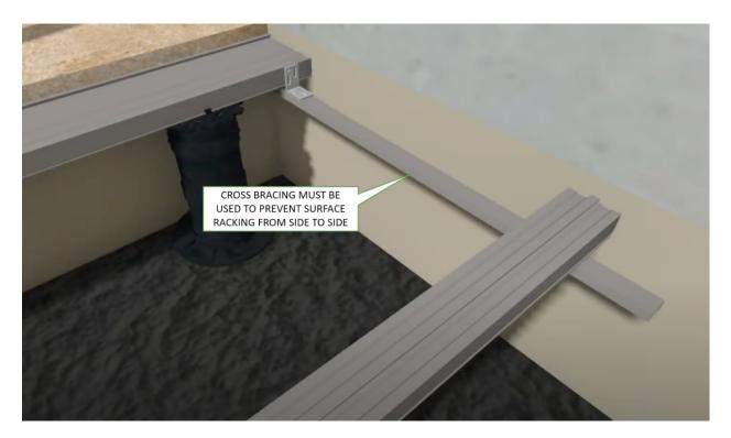
8. At this time, only attach the cross bracing to the first track and use one Mbrico tile as a spacer to align your second track. The grooved edge of the tile will be received by the male spline on the tracks.
